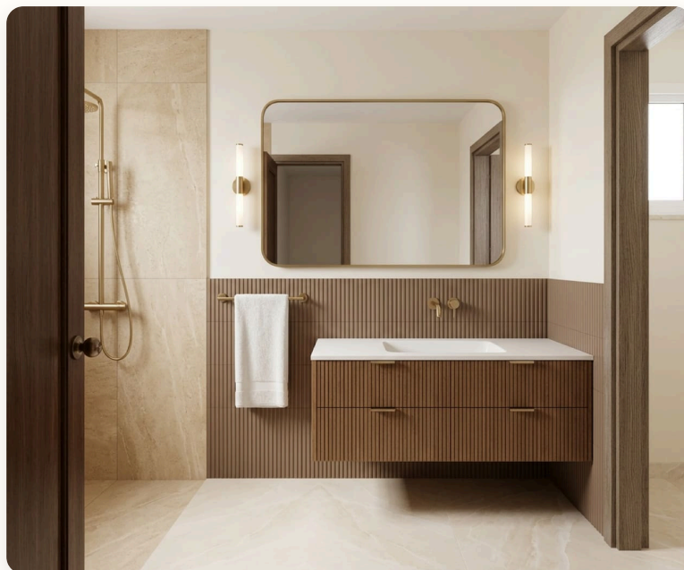
After (idea 1) — a floating 60 × 18 in mocha vanity, white quartz top, one wide basin, a brass-framed mirror with a light on each side, mocha ribbed tiles behind.
